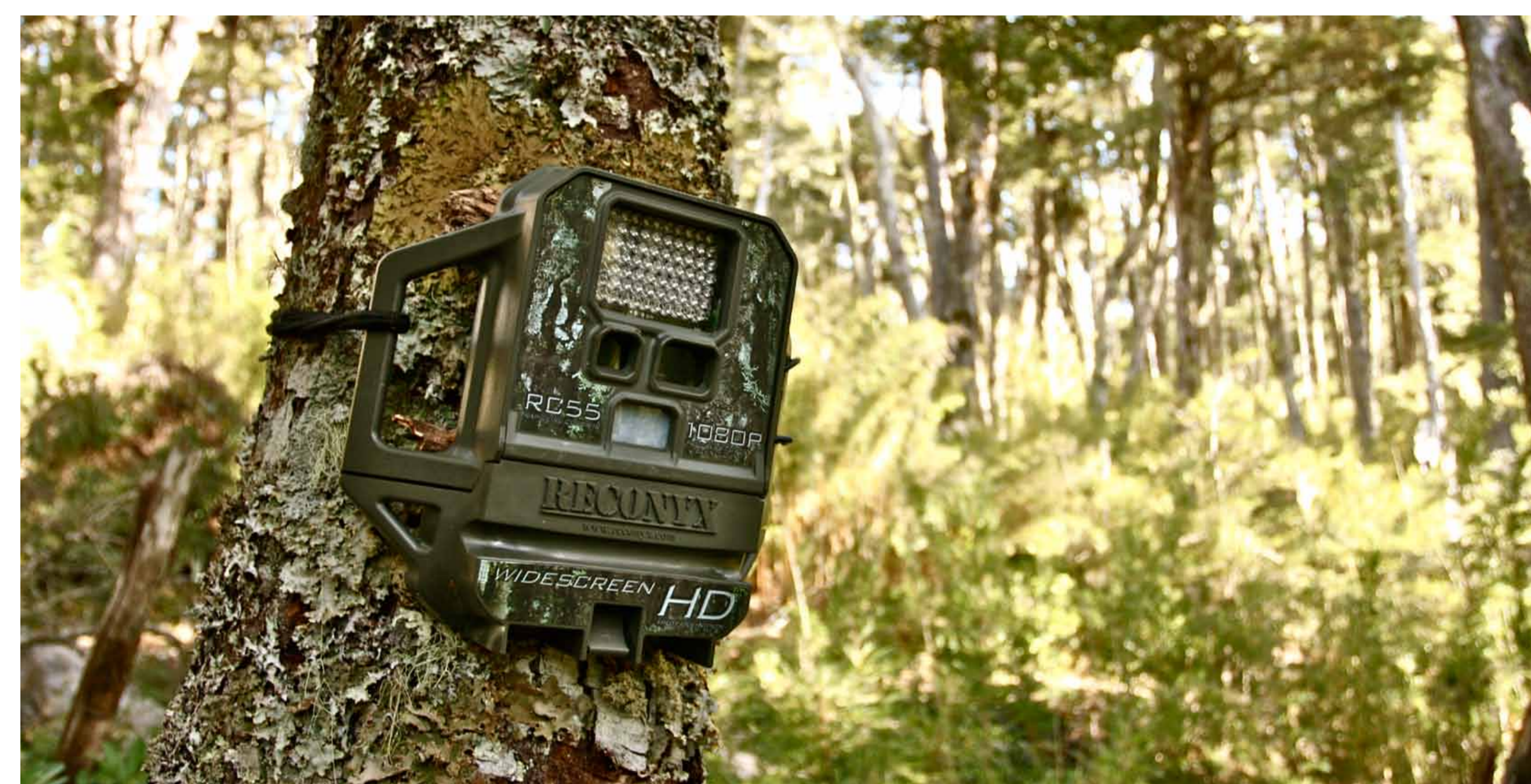
Digital scouting camera used for locating and recording the shy and elusive mammals of the Chilean temperate rainforest.
